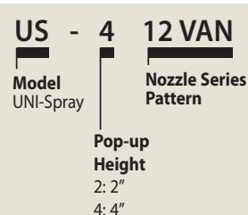
This specifies a UNI-Spray body with a 4" (10,3 cm) pop-up height; 12 foot (3,6 m) variable arc nozzle (VAN)
